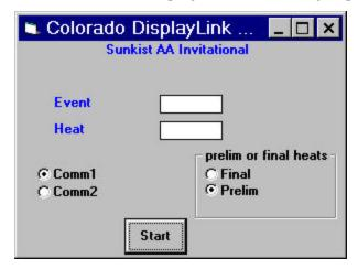
Connect the scoreboard PC to COM port #2 of your meet management PC using a null modem cable and click on the Start button. Meanwhile, the scoreboard operator can select and display data by requesting that data by event and heat using the Colorado-supplied scoreboard operations program shown below:
